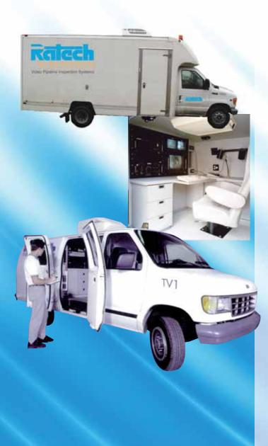
The Ratech Visu-Van<sup>®</sup> is a high quality self-contained, all weather television inspection vehicle for sewer and pipe inspection. It combines a low maintenance, high performance and dependable method of pinpointing sewer problems without the costly trial and error methods of excavation. It also gives you a state-of-the-art inspection tool to verify specifications, workmanship, alignment and grade information before final acceptance on new or reconditioned installations and projects.
